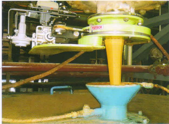
YUTECH CSD Pneumatic Control Valve Automatically Feeds Continuous Centrifugal Machine
